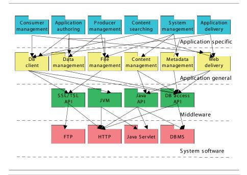
Figure 2 Software architecture
