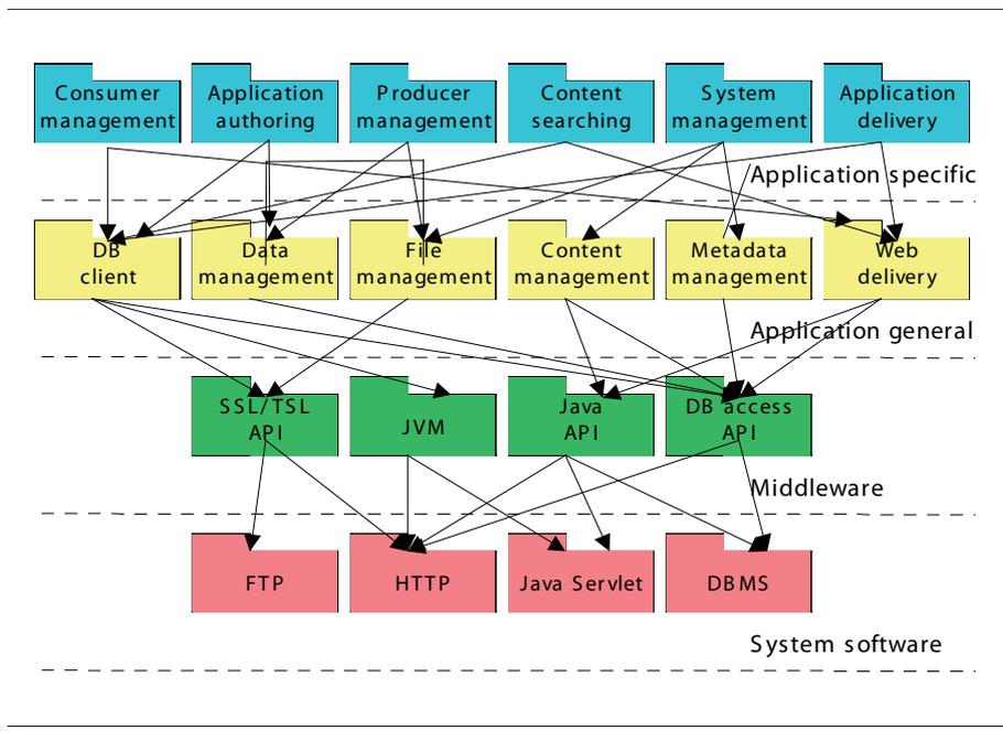
Figure 2 Software architecture
